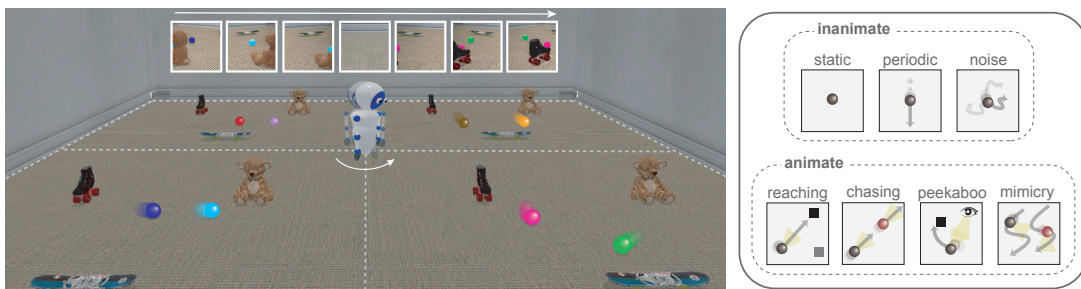
Figure 1: Virtual environment. Our 3D virtual environment is a distillation of key aspects of real-world environments. The curious agent (white robot) is centered in a room, surrounded by various external agents (colored spheres) contained in different quadrants, each with dynamics that correspond to a realistic inanimate or animate behavior (right box). The curious agent can rotate to attend to different behaviors as shown by the first-person view images at the top. See https://bit.ly/31vg7v1 for videos.
